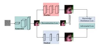
Figure 1: Framework of data-free knowledge distillation for image super-resolution.
