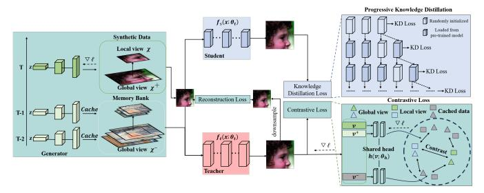
Figure 2: Framework of data-free knowledge distillation based on contrastive learning. The generator is trained with reconstruction loss, Contrastive Loss, and adversarial loss to synthesize images that are similar to the original data. The student network is then obtained utilizing progressive distillation from the teacher network.
